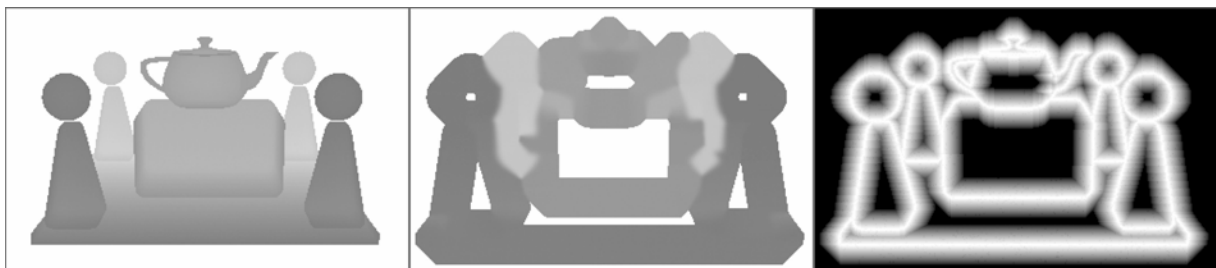
Figure 5: Individual channels (RGB) of the shadow map after preprocessing – original depth in red, nearest occluders in green, inversed distance to hard shadow boundary in blue (modified to be visible).
